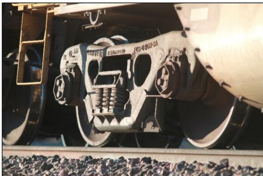
**Figure 1. Freight car side frame and wheels**
